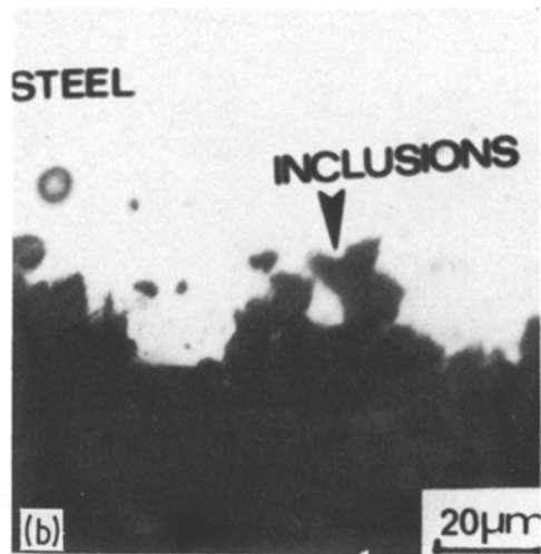
Figure 16 Photomicrographs showing the presence of inclusions in the used tabular alumina filter volume. (a) and (b) Optical micrographs of the top and bottom portions, respectively, of the filter. (c) Scanning electron micrograph showing the inclusion attachment to the filter grain (sample etched with bromine-methanol).
